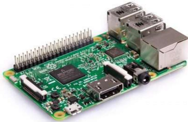
Figura 4-6: Raspberry Pi 3 Modelo B<sup>2</sup>
