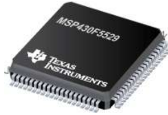
Figura 4.2: Microcontrolador MSP430F5529 de Texas Instruments .
